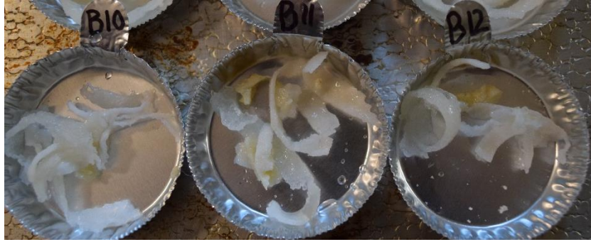
Figure 9. Image of 10 mm slices of No-Hide Beef 60 dog chews after immersion for 8 hours in simulated canine gastric juice. Samples showed strong degradation, softening, color loss, particle formation and unraveling.
