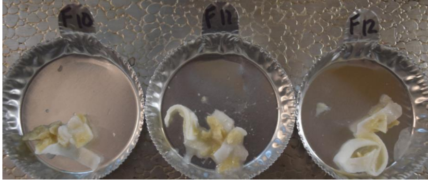
Figure 11. Image of 10 mm slices of No-Hide Beef 60 dog chews after immersion for 8 hours in simulated canine intestinal juice. Samples showed very good degradation, softening, color loss, particle formation and unraveling.
