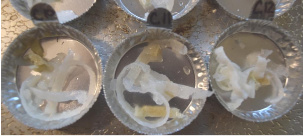
Figure 13. Image of 10 mm slices of No-Hide Chicken 45 dog chews after immersion for 8 hours in simulated canine gastric juice. Samples showed degradation, softening, particle formation, unraveling and color loss.
