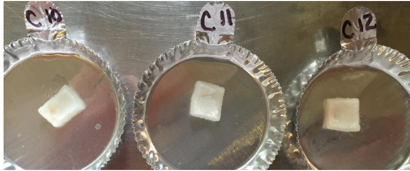
Figure 21. Image of 10 mm slices of Rawhide dog chews after immersion for 8 hours in simulated canine gastric juice. Samples showed some degradation, some softening and color loss.
