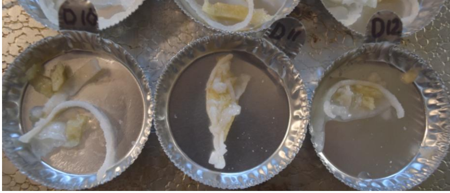
Figure 17. Image of 10 mm slices of No-Hide Chicken 60 dog chews after immersion for 8 hours in simulated canine gastric juice. Samples showed strong degradation, softening, particle formation, unraveling and color loss.
