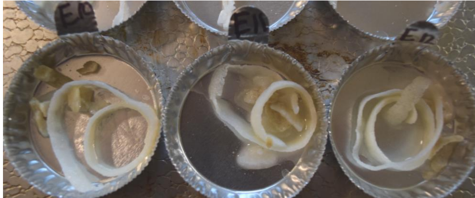
Figure 7. Image of 10 mm slices of No-Hide Beef 45 dog chews after immersion for 8 hours in simulated canine intestinal juice. Samples showed good degradation, softening, color loss, particle formation and unraveling.
