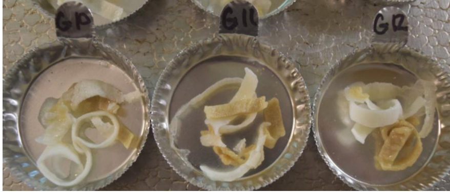
Figure 15. Image of 10 mm slices of No-Hide Chicken 45 dog chews after immersion for 8 hours in simulated canine intestinal juice. Samples showed degradation, softening, particle formation, unraveling and color loss.
