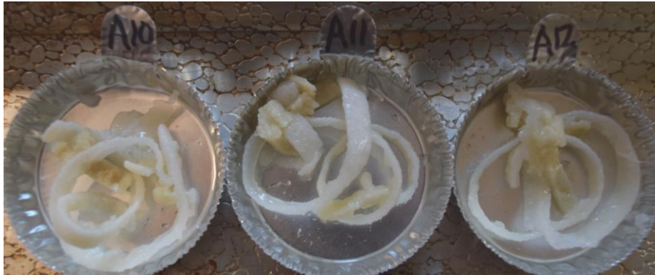
Figure 5. Image of 10 mm slices of No-Hide Beef 45 dog chews after immersion for 8 hours in simulated canine gastric juice. Samples showed degradation, softening, color loss, particle formation and unravelling.
