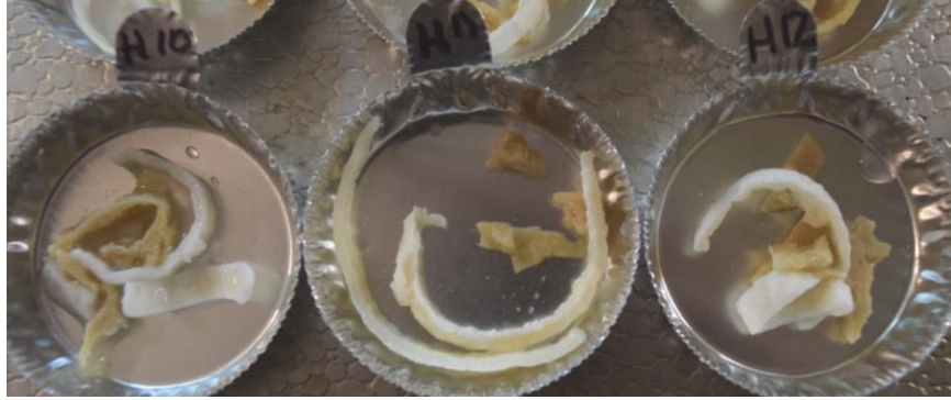
Figure 19. Image of 10 mm slices of No-Hide Chicken 60 dog chews after immersion for 8 hours in simulated intestinal juice. Samples showed strong degradation, softening, particle formation, unraveling and color loss.
