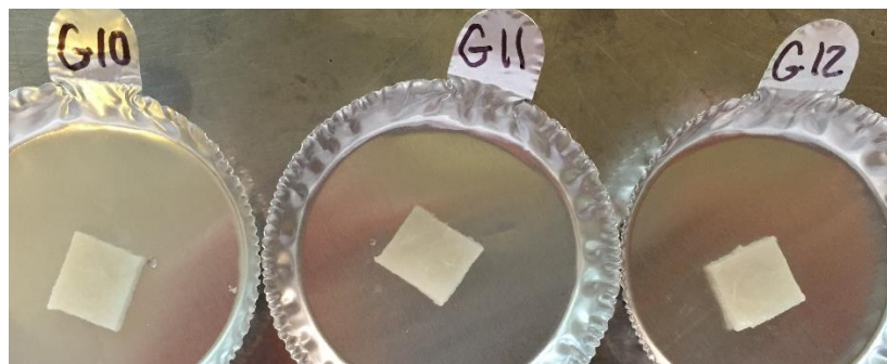
Figure 23. Image of 10 mm slices of Rawhide dog chews after immersion for 8 hours in simulated canine intestinal juice. Samples showed little degradation, some softening and color loss.
